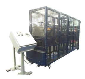
The RWM CFTMA (or Caster and Floor Truck Manufacturing Association) machine is a swivel test machine that tests the endurance of swivel casters by rotating them back and forth under load continuously. The machine swivels the caster under a programmed load and moves a small distance before rotating and traveling the opposite direction.
