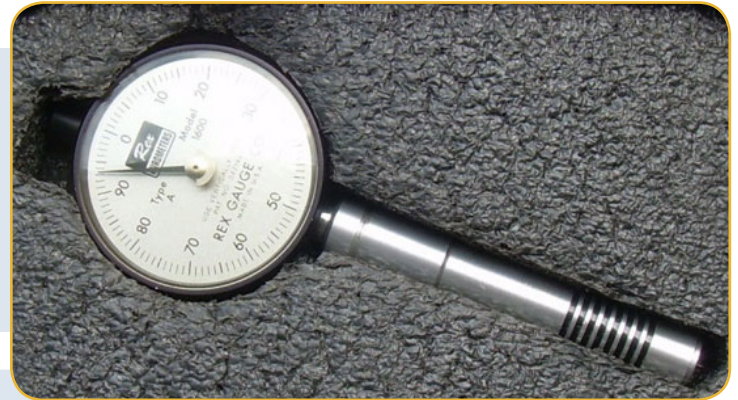
Figure 3. Shore A Durometer
