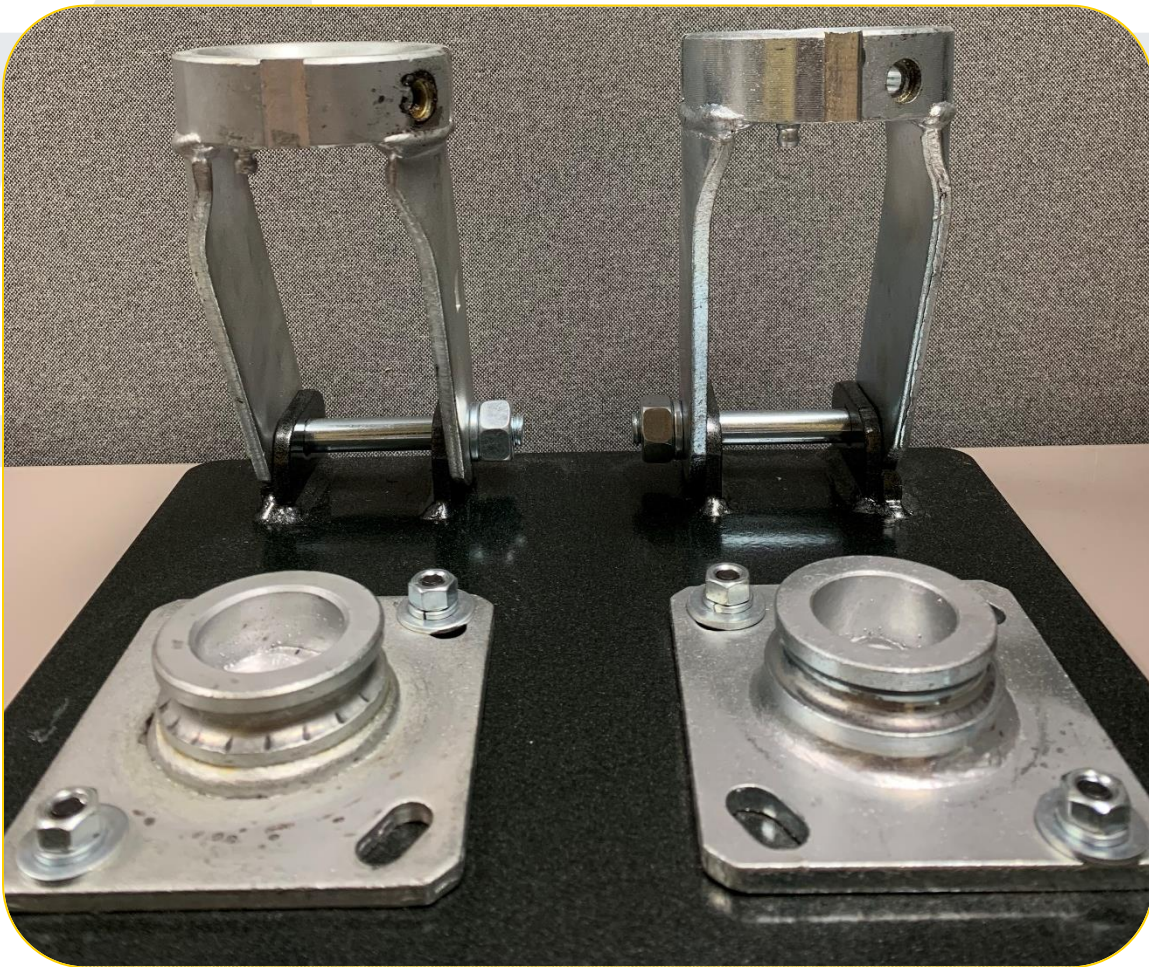
Images compare the non-heat treated caster (left) and the heat treated caster (right)
