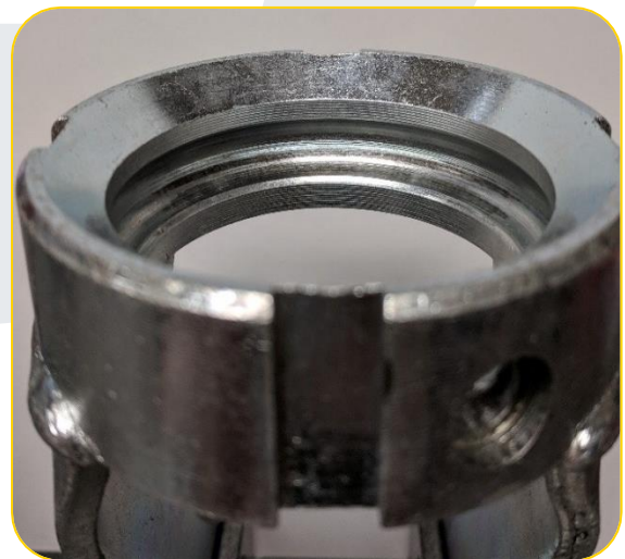
RWM 65 Series heat treated Raceway after 2 hour obstacle test
