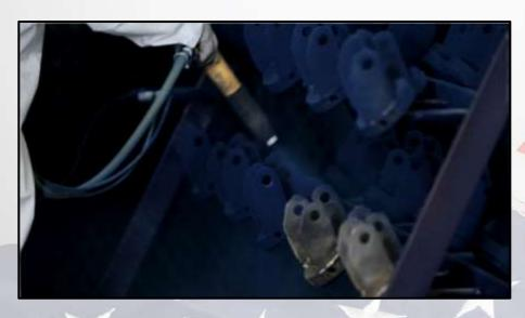
RWM was the first U.S. caster manufacturer to offer powder coating as a standard on our heavy duty Kingpinless products. Powder coating extends the lifespan of the caster rig by providing a stronger barrier against corrosives and everyday use in the workplace. Powder coating is a superior protective finish to the silver zinc plating prevalent in the market and is offered at no additional charge from RWM. Check out our new video showcasing our powder coating capabilities.
