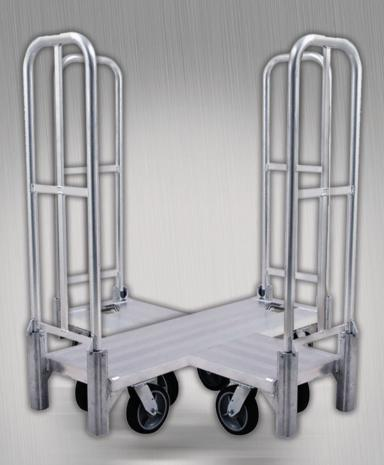
Our Titan Bulk Delivery Truck saves time, space and money for all route delivery companies. The Titan BDT offers maximum maneuverability, zero turn radius and has a 1200 pound capacity. Heavy duty aluminum welded construction adds superior strength and durability for a long lasting product.
