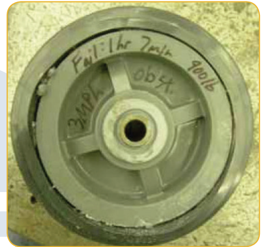
Figure 4: Typical Failure during an Obstacle Test
