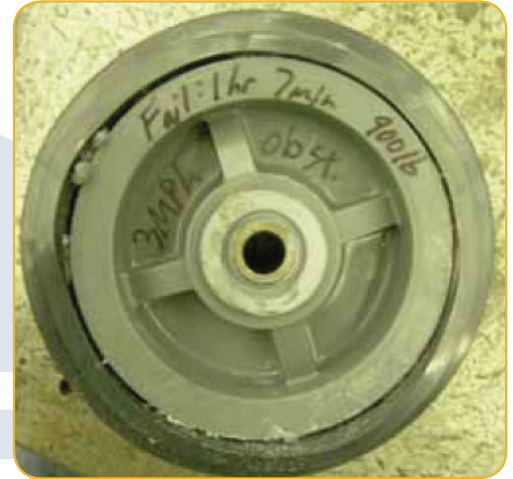
Figure 4: Typical Failure during an Obstacle Test
