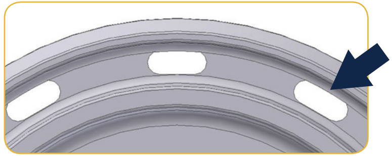
Figure 1. Example of a mechanical bond "pass through" hole.
