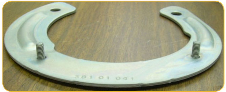
Figure 3. An example of a Zinc Nickel plated part
